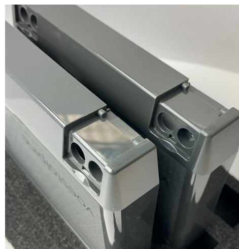
Fig. 2: Molded ABS plastic parts, manufactured with TiN-coated (left) and CHROME-X®-coated (right) tools
